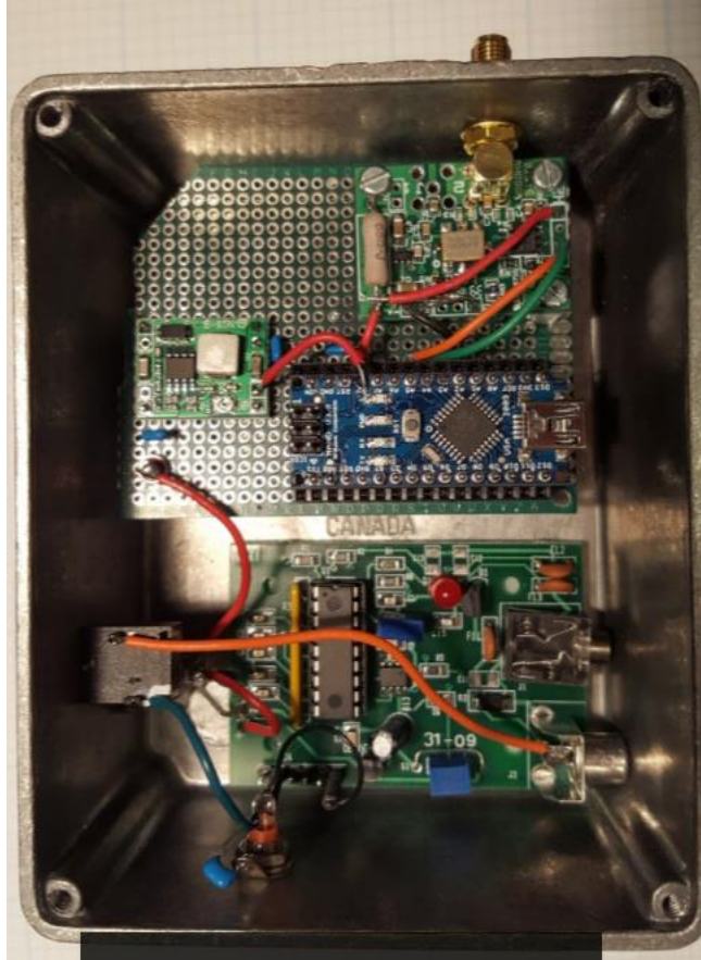
Figure 6. The signal source is enclosed with a KT-4 beacon keyer in a Hammond box with jacks that bring in 12V, an RF sample voltage, and the keying line. The RF is brought out via the daughterboard SMA and an RCA jack is used for external metering of the RF sample.
